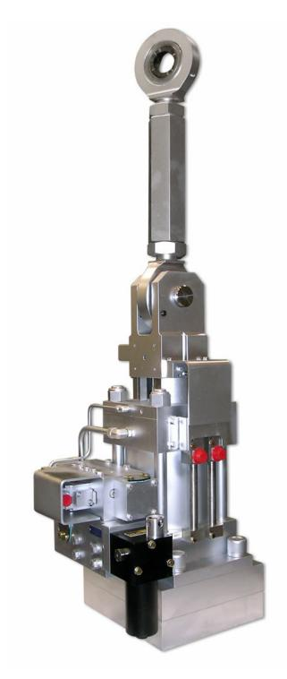
Used for Inlet Guide Vane (IGV) positioning and control of industrial or utility large frame gas turbines, the 8277 Series Severe Service Hydraulic actuators will force the IGV's closed in the event of a turbine trip. Ruggedized and proven to withstand the harsh control conditions associated with high dither rates.
