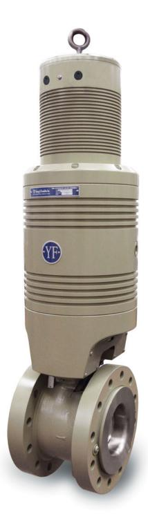
The Young & Franklin 8655 Series Electric Stop/Ratio Valves are designed to regulate fuel pressure and provide rapid fuel shutoff capability. Fail Safe to closed position is accomplished by the use of two torsion springs. The actuator is suitable for fuel modules in Class 1 Div 2 Hazardous Locations.
